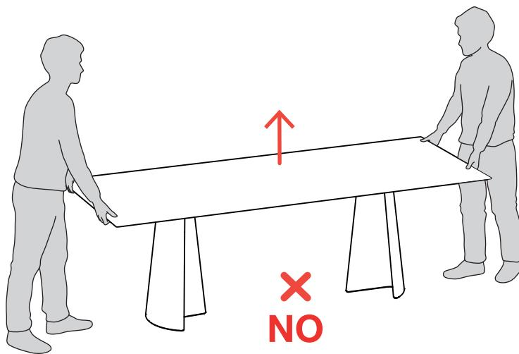
!! After assembly, do not lift or move the table by holding it from the top.
