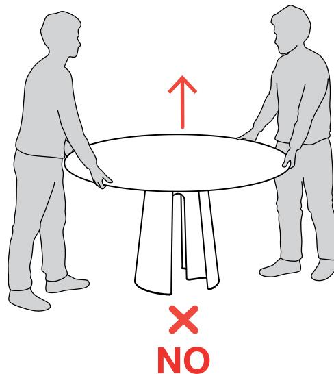
!! After assembly, do not lift or move the table by holding it from the top.
